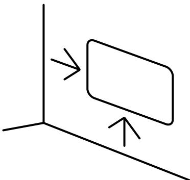
**2** Select a suitable wall for your heater, ensuring there is at least a 4½" clearance between the heater and the nearby walls, ceiling, and floor. Additionally, place the heater in a location where the cord can reach an outlet for power.
